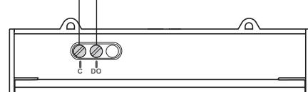
**en** The digital output is polarity-independent.
