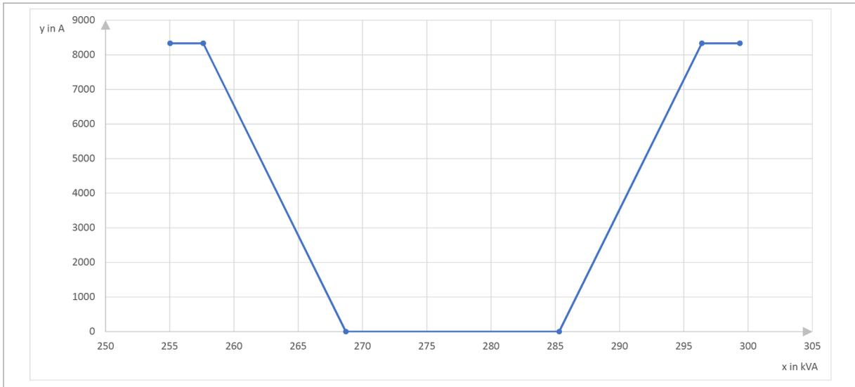
Current/reactive power characteristic curve for ranges in which reactive power compensation occurs.
