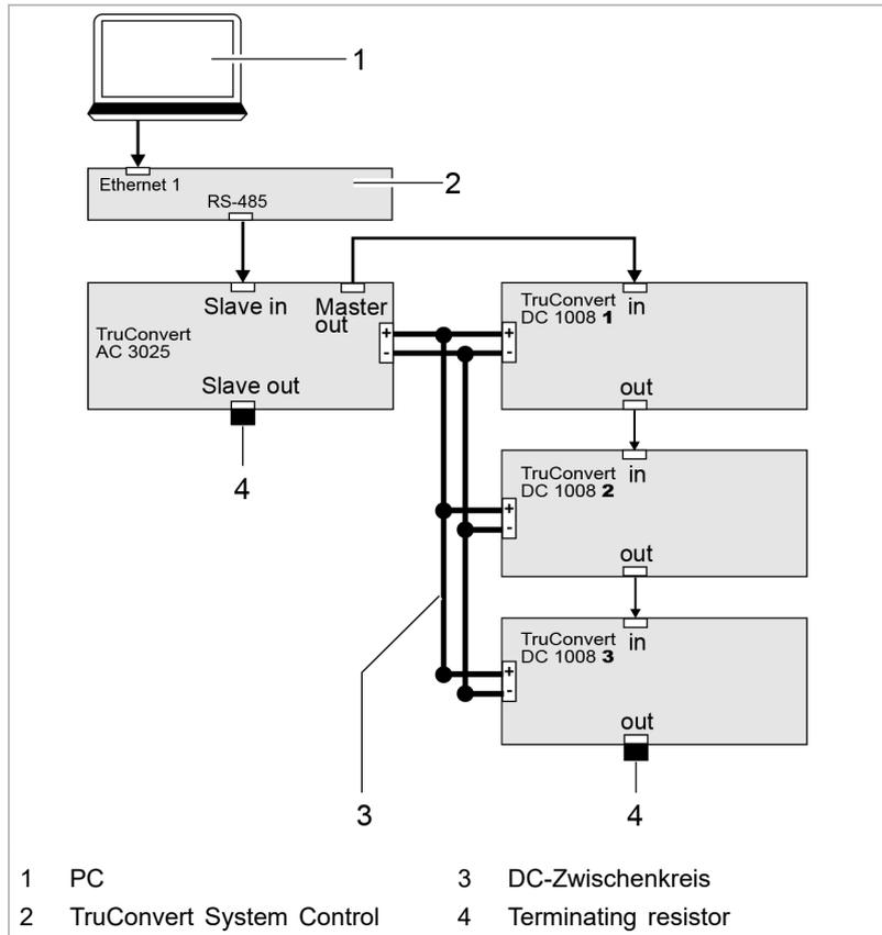
One TruConvert System Control controls one TruConvert AC 3025 and m x TruConvert DC 1008
