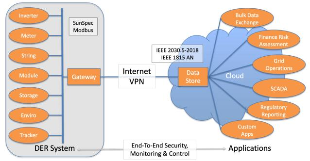
The specifications are intended to reduce the cost of system implementation through standardization. By enabling applications to be written using a single, standardized view of solar plant components, independent of component manufacturer and model, devices can maximize cost efficiencies and potential deployment possibilities through interoperability with other applications and devices.
